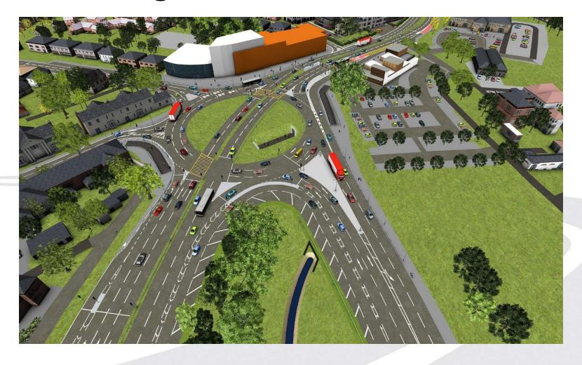
Otherwise known as a throughabout, traffic would be able to travel straight between Essex Yeomanry Way and Parkway through the centre of the junction without using the roundabout. Traffic travelling to other arms of the junction would use the roundabout. Traffic signals would be used to manage traffic flows and priority.
