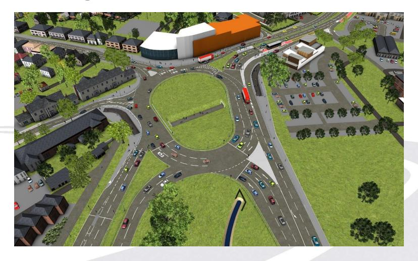
The existing roundabout would be enlarged into the floodplain, creating a larger circulatory. The approach lanes on Parkway would also be widened. Traffic flows would be managed by traffic signals
