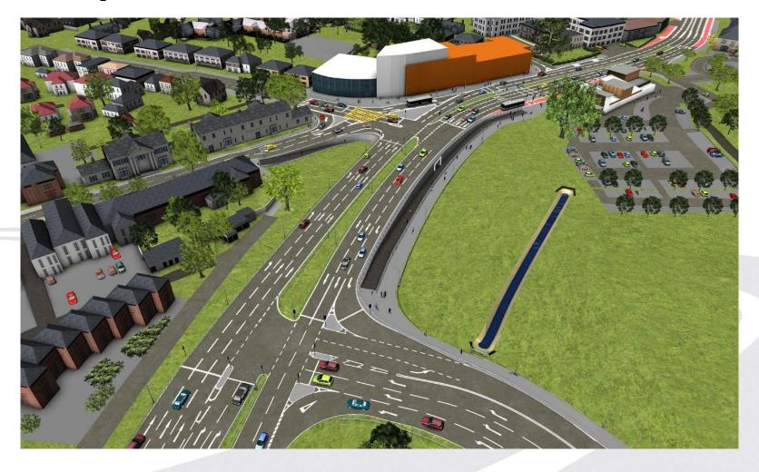
Two new T-junctions created – one linking Essex Yeomanry Way and Chelmer Road, and the other linking Essex Yeomanry Way/Parkway and Van Diemans Road/Baddow Road. Traffic signals would be used to control traffic flow at the junctions.
